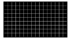
This pattern displays a series of horizontal and vertical straight white lines that forms a grid of 16 x 9 squares of the same size for 1080i and 720p, 12 x 9 squares for 480p and NTSC.
