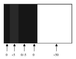
The PLUGE (stands for Picture Line-Up Generation Equipment) pattern is divided into two halves.
