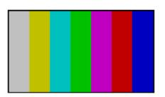
Seven equal width vertical color bars are displayed at 75% amplitude, 100% saturation in the order from left to right: White, Yellow, Cyan, Green, Magenta, Red, and Blue.
