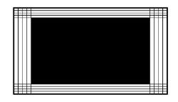
The Overscan-Bounce pattern consists of 4 horizontal lines on the top and bottom edge of the screen and 4 vertical lines at the left and right edge of the screen. These lines mark 2.5%, 5%, 7.5%, and 10% of the width and height of the screen. The background of the screen alternates between black and white.
