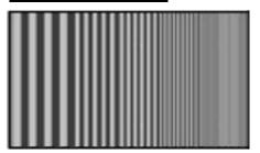
The MULTIBURST pattern displays five frequency bands of progressively higher frequency from left to right. The following frequencies are displayed: 2.32MHz, 4.64MHz, 6.19MHz, 9.28MHz, and 18.56MHz for 1080i / 720p formats; 1.16MHz, 2.32MHz, 3.09MHz, 4.64MHz, and 6.19MHz for 480p; 1.16MHz, 1.55MHz, 2.32MHz, 4.64MHz for NTSC format.
