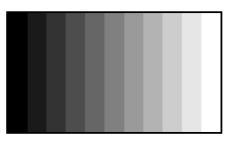
The STAIRCASE pattern displays equal-width vertical bar steps of increasing luminance from left to right.
