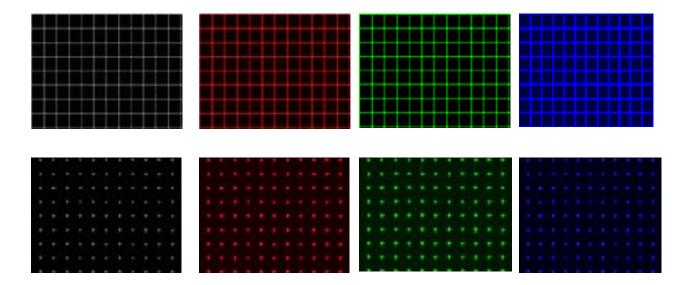
The CROSS HATCH patterns display a series of horizontal and vertical straight white lines that forms a grid of 12 x 8 squares of the same size.
